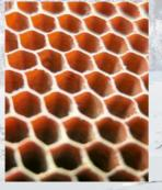
Nomex is extra light, aviation grade Kevlar-reinforced honeycomb construction with top-class power transmission features. Due to the dynamic action of the construction it is used especially in race skis.
